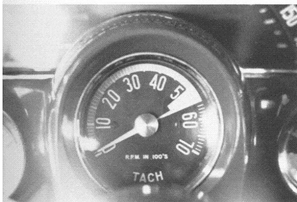
From the top: Tach used in '58 for high performance, high-lift-cam engines, RPO 469 and RPO 579. Base tach, part number 1548803, used for 1959 cars. Base tach for 1960-1962 Corvettes, this same tachometer also being used on all hydraulic-lifter engines (RPO 469 and RPO 579) that year as well.
