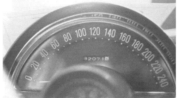
Above: Speedometer for '58. Kilometer-graduated speedometer in '59 car, destined for Switzerland. Below: Instruments for 1958-'59 cars had round-tipped needles, for 1960-'62 they were tapered and sharp-tipped.
